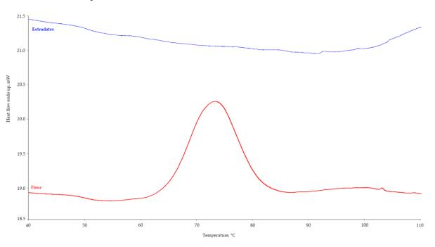
**Figure 2.** DSC curves for the flour mixture before extrusion (red curve) and extrudate sample (blue curve).
