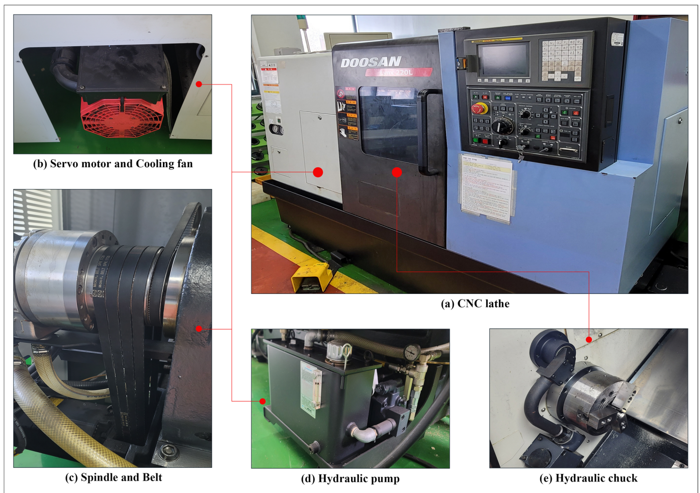
Figure 2. Major components of vibration in CNC lathes. (a) CNC lathe used in the experiment; (b) servomotor used to drive the spindle; (c) belt and main spindle connected to the servomotor to transmit power; (d) hydraulic pump used to operate the hydraulic chuck and tailstock; and (e) hydraulic chuck to hold the workpiece.
