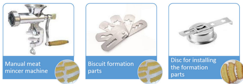
Figure 2. Manual meat mincer machine, modified for biscuit formation.
