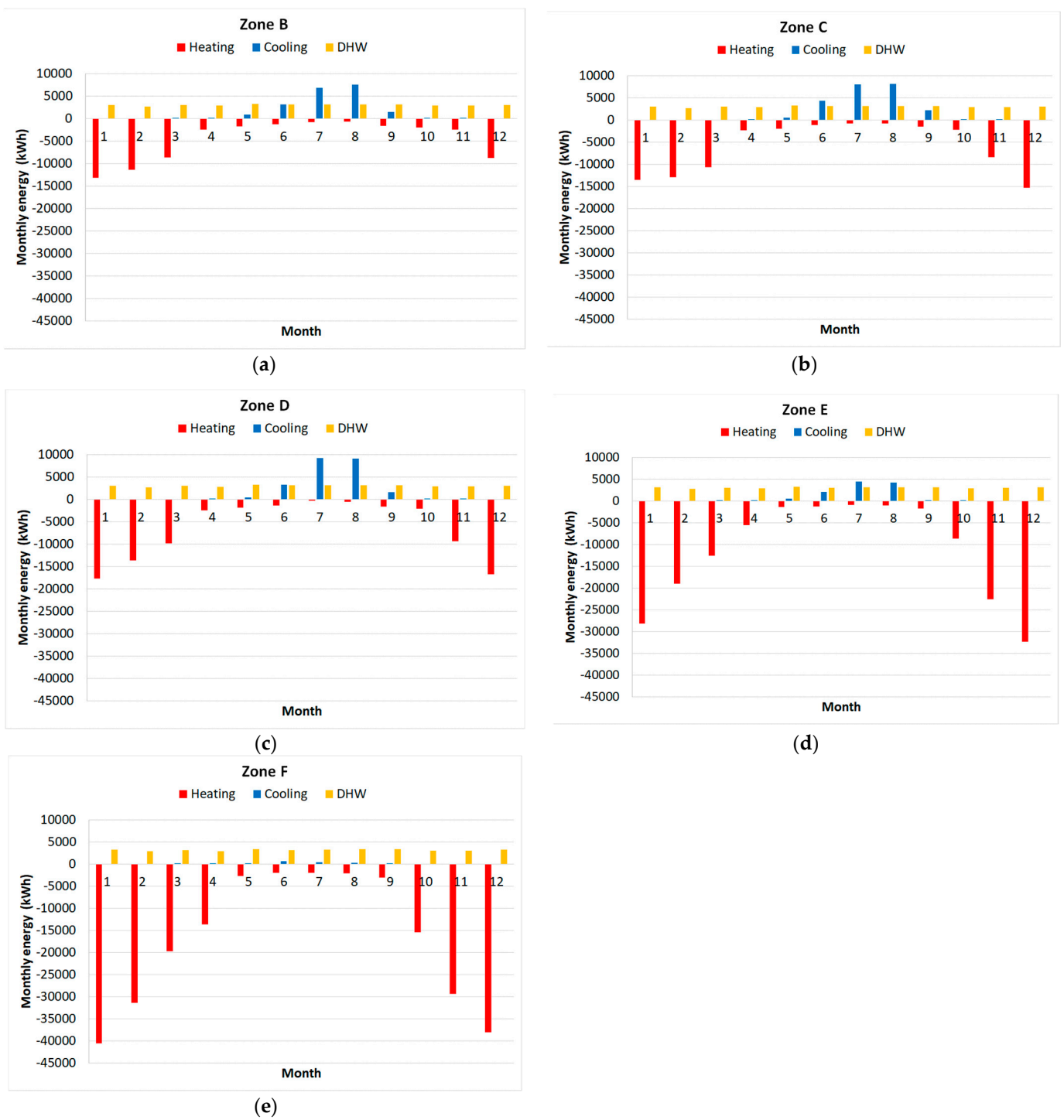
Figure 2. Monthly energy needs for heating, cooling and DHW of the condominium for the base case for the different climatic zones (a–e).
