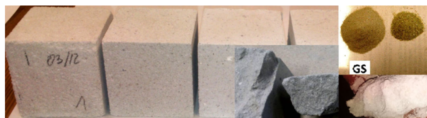
Figure 4. Silicate brick a brick with dimensions of 5 \times 5 \times 5 cm modified with recycled glass sand and a break through the structure of the brick modified by 90 wt% glass sand (GS).
