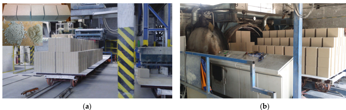
Figure 29. Example silicate brick production line (Ludynia, Poland); (a) pressing process under pressure of fresh silicate mass; (b) autoclaving process of pressed and formed silicate brick under pressure.
