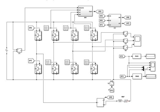
Figure 9. The model of the symmetry device based on the PI controller in MATLAB/Simulink [41].
