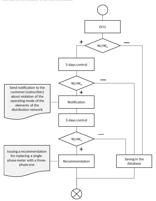
Figure 2. Algorithm for monitoring energy consumption using smart electricity meters.
