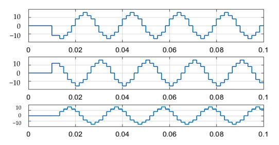
**Figure 11.** Phase voltage waveform at  $150^{\circ}$  [41].
