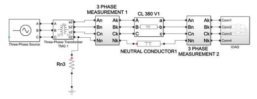
Figure 5. Model of a section of the urban electricity distribution network with 148 consumers connected.
