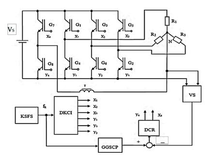
Figure 6. Diagram of the implementation of the symmetry device.
