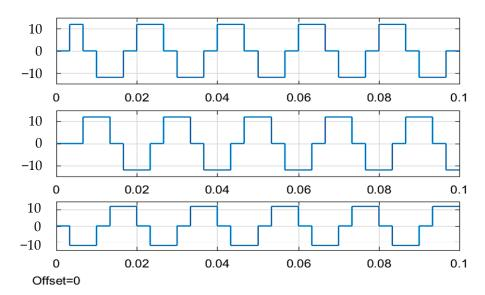
**Figure 10.** Phase voltage waveform at 120° [41].
