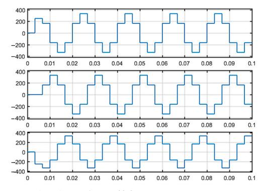
**Figure 12.** Phase voltage waveform at  $180^{\circ}$  [41].
