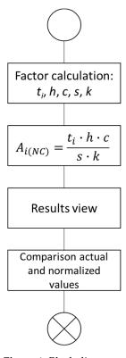
Figure 1. Block diagram of the prediction algorithm.
