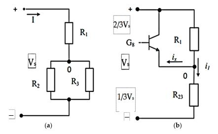
**Figure 7.** Initial substitution diagram without symmetry (**a**) and equivalent substitution diagram with symmetry (**b**).
