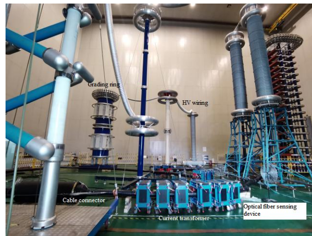
Figure 6. Wiring diagram for partial discharge testing of optical fiber sensing cable.
