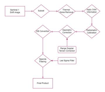
Figure 2. Pre-processing workflow of SAR images.
