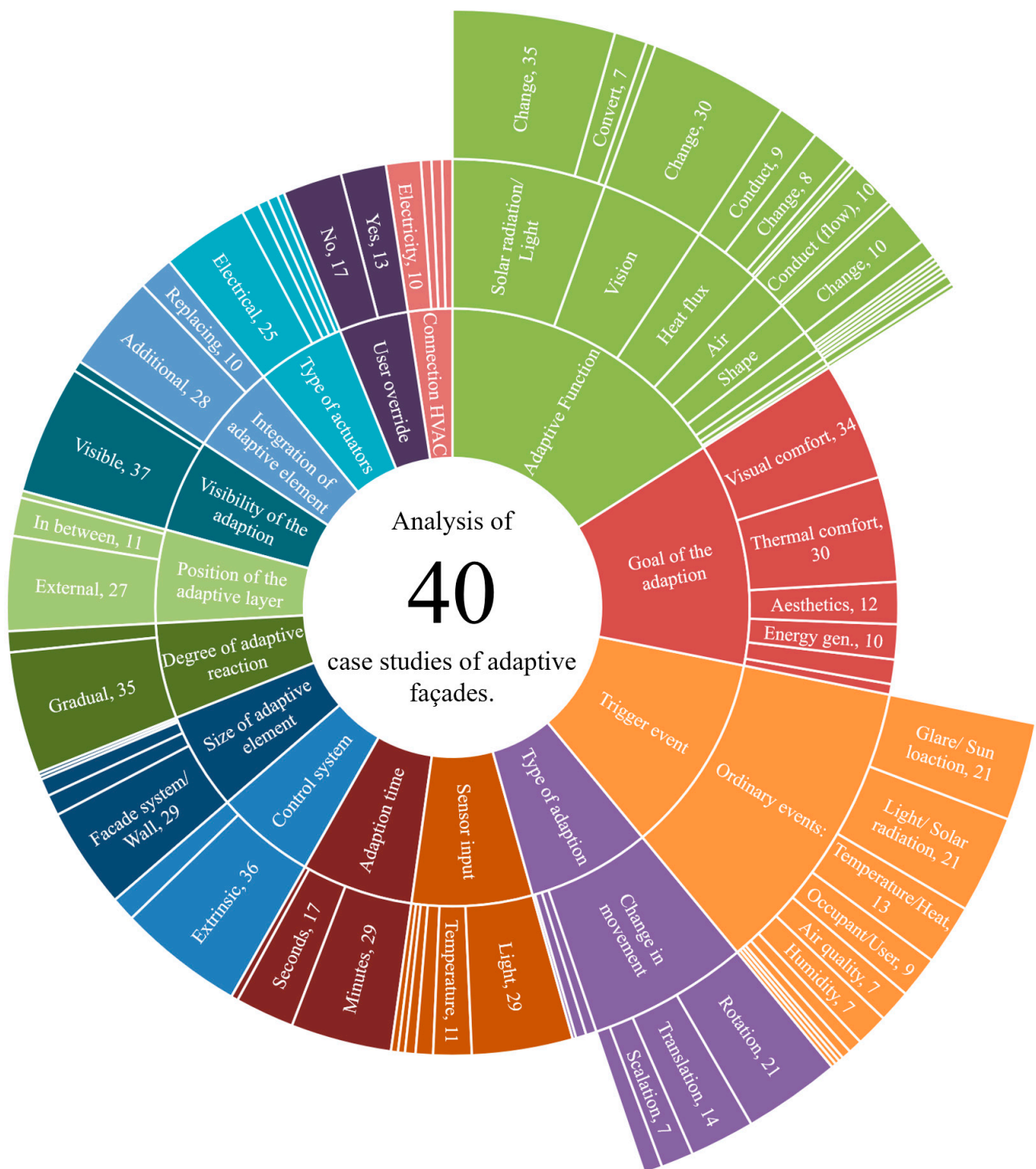
Figure 17. Assigning 40 AF case studies to the design parameters (sorted by frequency), from [24].
