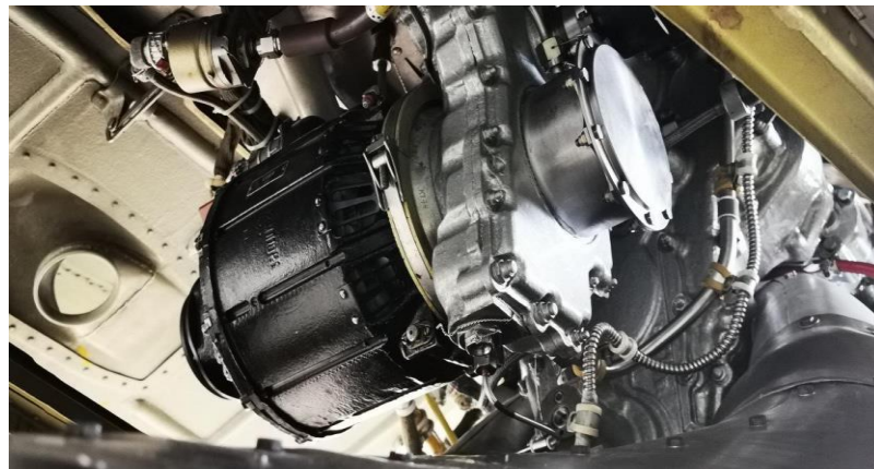
Figure 1. GT16PCz8 generator installation.
