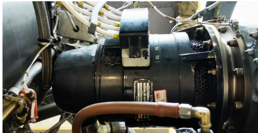
Figure 4. Generator integrated on the engine.
