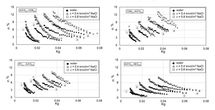
**Figure 8.** The distribution of gas hold-up as a function of a number of gas flow Kg for different superficial gas velocity  $w_{\rm og}$ :  $1-w_{\rm og} = 1.706 \times 10^{-3}$  m/s,  $2-w_{\rm og} = 3.413 \times 10^{-3}$  m/s,  $3-w_{\rm og} = 5.119 \times 10^{-3}$  m/s,  $4-w_{\rm og} = 6.826 \times 10^{-3}$  m/s.
