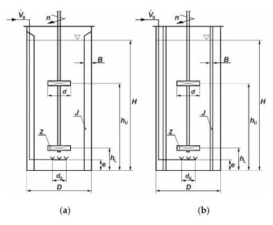
**Figure 1.** Geometrical parameters of the vessel with: (a) four planar standard baffles; (b) 24 vertical tubular baffles located on the circuit.
