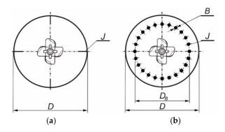
Figure 2. Located baffles inside vessel; (a) four planar standard baffles; (b) 24 vertical tubular baffles located on the circuit.
