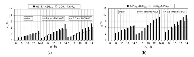
**Figure 9.** Dependence of  $\varphi = f(n)$  for two different impeller configurations A315<sub>(L)</sub>-CD6<sub>(U)</sub> or CD6<sub>(L)</sub>-A315<sub>(U)</sub> and for three different gas–liquid systems for superficial gas velocity  $w_{og}$ : (a) 1.706 ×  $10^{-3}$  m/s, (b) 5.119 ×  $10^{-3}$  m/s.
