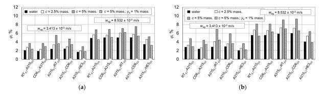
**Figure 4.** Dependence of  $\varphi$  = f(configurations of impeller); standard planer baffles, (a) n = 10 1/s; (b) n = 12 1/s.
