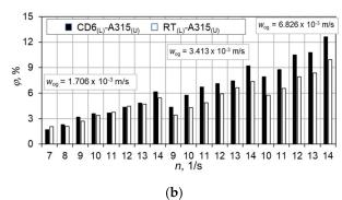
**Figure 7.** Dependence of  $\varphi = f(n)$  for two different impeller configurations CD6<sub>(L)</sub>-A315 <sub>(U)</sub> or RT<sub>(L)</sub>-A315<sub>(U)</sub> and for two different gas–liquid systems: (a) air–water system, (b) air–aqueous solution NaCl of concentration c = 0.8 kmol/m<sup>3</sup>.
