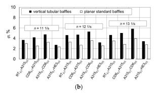
**Figure 11.** Dependence of  $\varphi$  = f(configuration of impellers), for different n;  $w_{\text{og}} = 3.413 \times 10^{-3} \text{ m/s}$ ; (a) water; (b) aqueous sucrose solution c = 2.5% mass.
