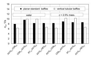
**Figure 10.** Dependence of  $n_{\rm cr}$  = f(configurations of impeller);  $w_{\rm og}$  = 3.413 × 10<sup>-3</sup> m/s.
