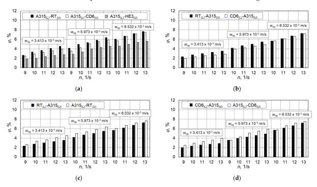
**Figure 3.** Dependence of  $\varphi = f(n)$  for different configurations of impeller; standard planer baffles, c = 2.5% mass. (a) the effect of the upper impeller type; (b) the effect of the lower impeller type; (c,d) the effect of replacement of two impellers on the shaft.
