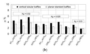
**Figure 12.** Dependence of  $\varphi$  = f(configuration of impellers), for different Kg;  $w_{og}$  = 3.413 × 10<sup>-3</sup> m/s; (a) water; (b) aqueous sucrose solution c = 2.5% mass.
