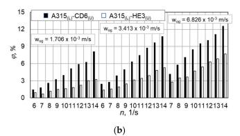
**Figure 6.** Dependence of  $\varphi = f(n)$  for two different impeller configurations A315<sub>(L)</sub>-CD6<sub>(U)</sub> or A315<sub>(L)</sub>-HE3<sub>(U)</sub> and for two different gas–liquid systems: (a) air–water system, (b) air–aqueous solution NaCl of concentration c = 0.8 kmol/m<sup>3</sup>.
