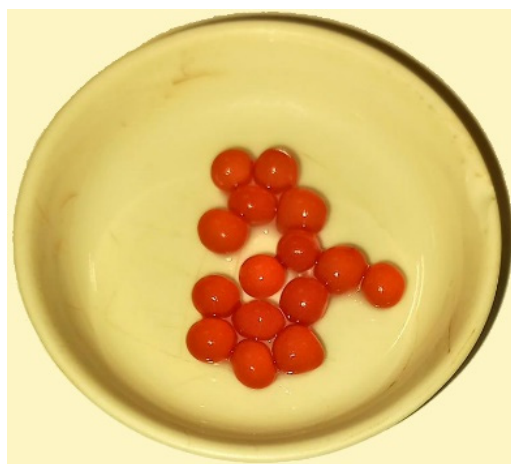
Figure 2. Calcium alginate beads with entrapped Rhodospseudomonas sp. cells.
