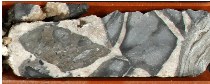
Figure 3. Core plug sample photo of angular breccia. Interval of cave roof collapse in the Loppa High region.
