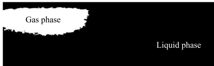
Figure 6. Image after image processing when the pressure is 0.15 MPa and tilted upward by 10°.
