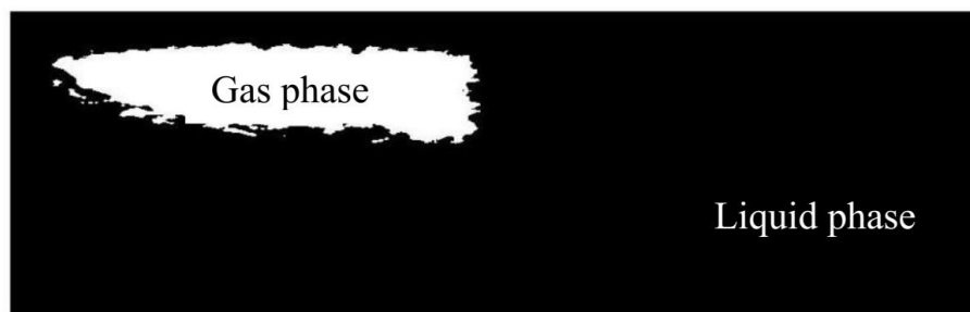
Figure 7. Image after image processing when the pressure is 0.2 MPa and tilted upward by 10°.
