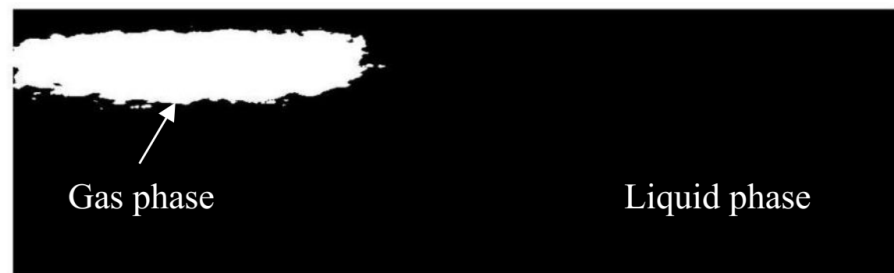
Figure 10. Image after image processing when the pressure is 0.15 \text{ MPa} and tilted upward by 20^\circ .
