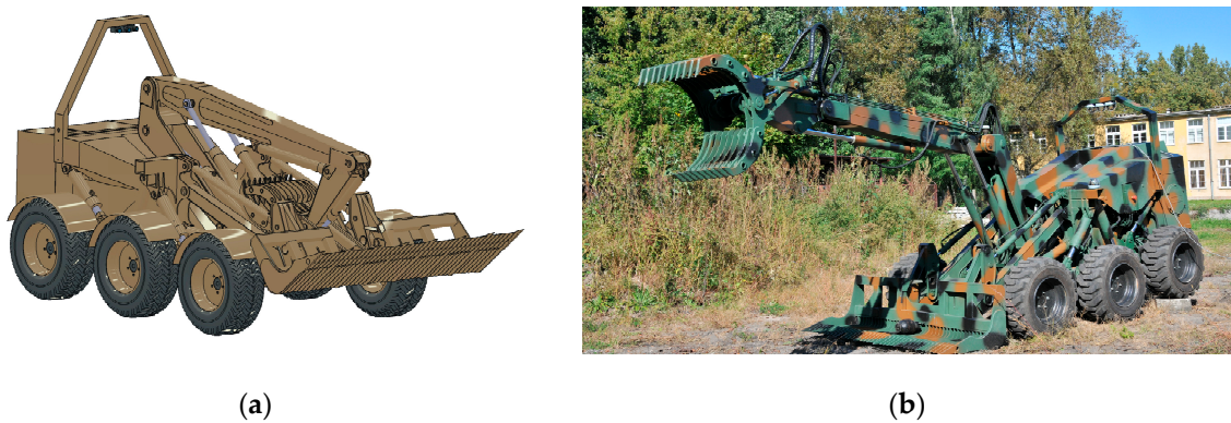
Figure 1. View of a 3D CAD model of the robot (a) and 6 \times 6 robot (b).
