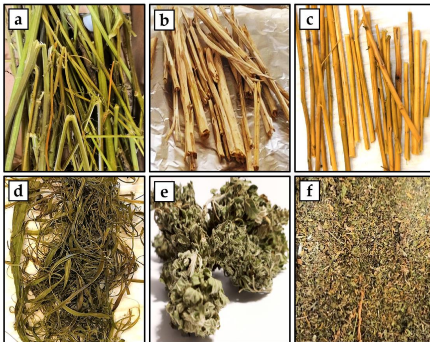
Figure 2. Pictures showing the different HBRs used in this study: stalks (a), the unretted hurds (b), the retted hurds (c), the fibers (d), the inflorescences (e) and the mix of leaves and inflorescences (f).
