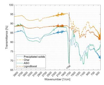
**Figure 6.** Typical attenuated total reflectance Fourier transform infrared spectroscopy (ATR-FTIR) spectra of the precipitated solids, char, ASO, and lignin. It can be noted that the char lacks the carboxyl peak at  $1706 \text{ cm}^{-1}$ .
