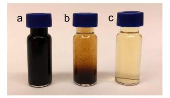
**Figure 2.** Hydrothermal liquefaction (HTL) product (**a**), acidified aqueous reaction product with precipitates (**b**), and filtrate of the acidified aqueous reaction products (**c**).
