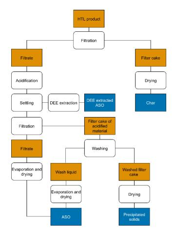
Figure 1. Schematic diagram of the fractionation of the reactor product.
