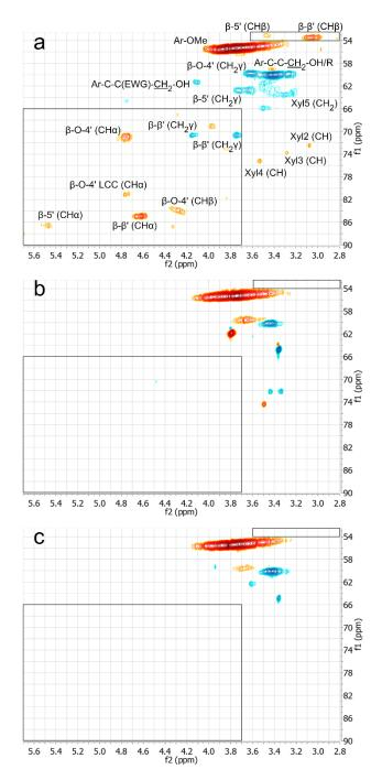
**Figure 3.** Inter-unit aliphatic region  $\delta_C/\delta_H$  52–90/2.8–5.7ppm of heteronuclear single quantum coherence spectroscopy (HSQC) spectra of the LignoBoost lignin (**a**), char (**b**) and precipitated solids (**c**). Notable inter-unit linkages and carbohydrate connections are marked with black squares [20]. EWG: electron withdrawing group. Xyl: xylan, with the corresponding carbon number. LCC: lignin–carbohydrate complex.
