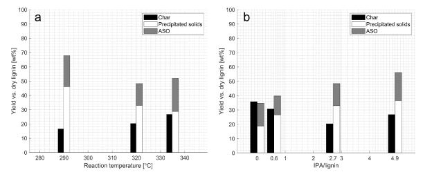
**Figure 4.** Yields obtained of the three product fractions vs. the dry lignin loaded in each reactor run: temperature series (**a**) and IPA series (**b**).
