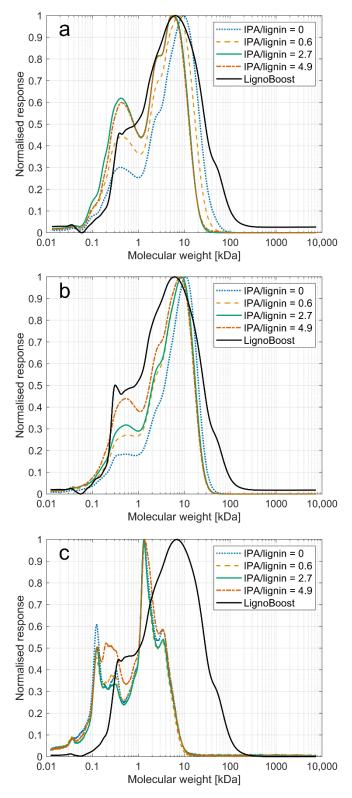
**Figure 5.** Gel permeation chromatography (GPC) chromatograms in the IPA series: char (**a**), precipitated solids (**b**), and ASO (**c**). These show that, with increasing IPA, the intensity of the low molar mass peak to the left increases for the char and precipitated solids.
