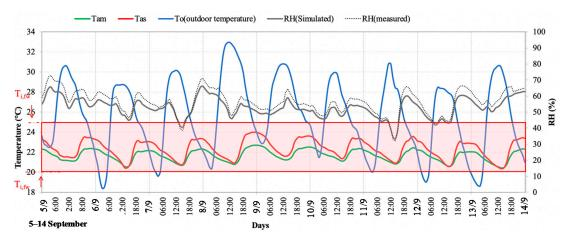
**Figure 5.** Daily profile of indoor temperatures at the current state of the building in free-running conditions during 5–14 September.
