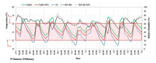
**Figure 8.** Daily profile of air temperature (T<sub>a</sub>) in the current state, after retrofit Ta (RI), and retrofit scenario with uninsulated floor on ground surface (RI-IGF) during the period 27 January–5 February.
