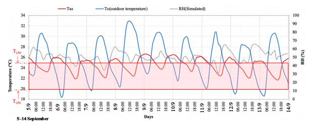
**Figure 7.** Daily profile of air and operative temperature after retrofit of the building in free-running conditions during 5–14 September.
