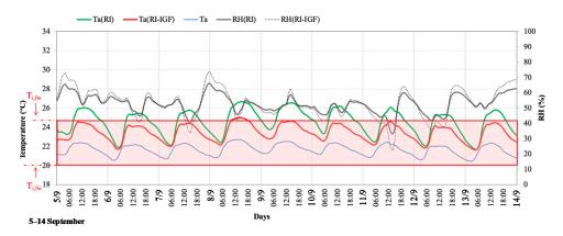
**Figure 9.** Daily profile of air temperature (T<sub>a</sub>) in the current state, after retrofit Ta (RI), and retrofit scenario with no insulated floor on ground surface (RI-IGF) during the period 5–14 September.
