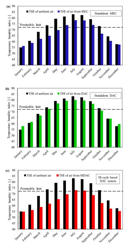
**Figure 8.** Analysis of proposed AC system options on monthly basis THI for Multan (Pakistan); (a) Stand-alone MEC system; (b) Stand-alone desiccant AC system; and (c) M-cycle based desiccant AC system.
