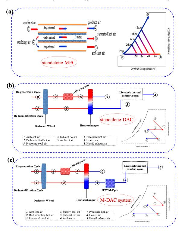
**Figure 2.** Proposed air-conditioning system options for this study: (a) stand-alone Maisotsenko-cycle evaporative cooling (MEC) system; (b) stand-alone desiccant air-conditioning (AC) system; and (c) M-cycle supported desiccant AC system.
