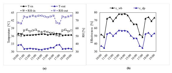
**Figure 4.** Analysis of experimental MEC system on hourly basis for 15 July for Multan (Pakistan): (a) outlet relative humidity and temperature; and (b) effectiveness.
