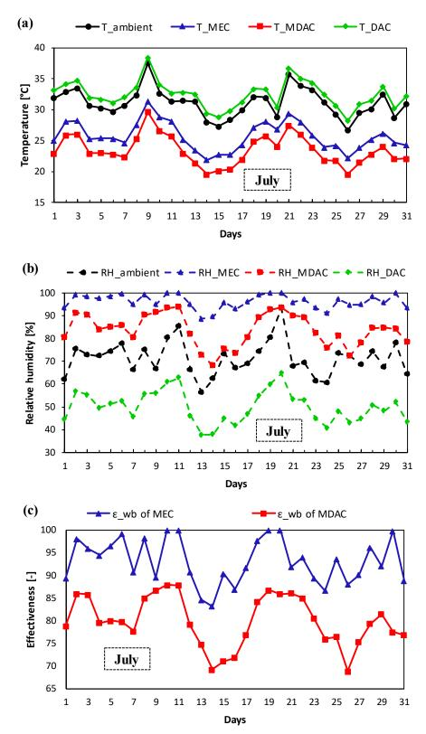
**Figure 5.** Analysis of proposed AC system options on daily basis for July for Multan (Pakistan); (a) outlet temperature; (b) relative humidity; and (c) effectiveness.
