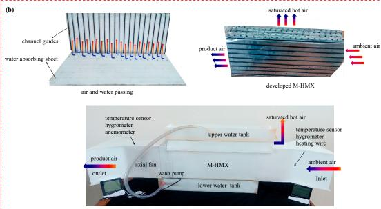
**Figure 3.** Schematic diagrams of M-cycle evaporative cooling system: (a) schematic diagram, and (b) pictorial representation of the experimental apparatus.
