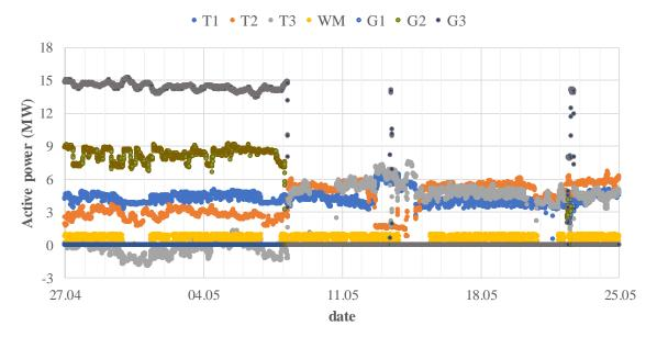
**Figure 3.** Active power of the high/medium (HV/MV) transformers T1, T2, and T3, welding machine (WM), and distributed generations G1, G2, G3 using the MV side measurements.
