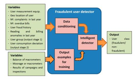
Figure 11. Functional structure of stage 3 of the system.
