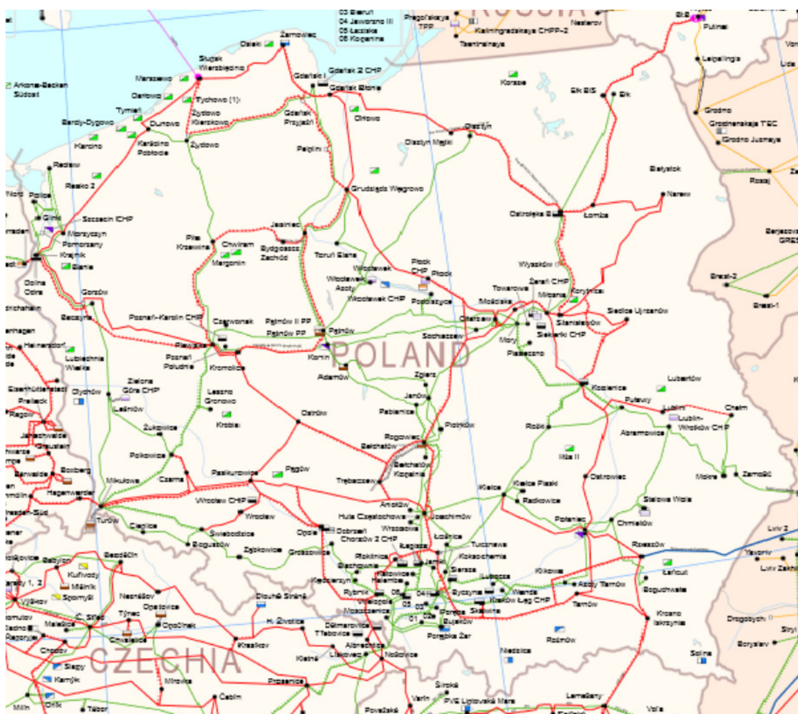
Figure 1. Map of the Polish National System of high voltage lines by the European Network of Transmission System Operators for Electricity, where the blue line marks 750 kV line, red 380–400 kV, yellow 300–330 kV and green 220–275 kV, the pink line means DC, gray lines are connection lines, and lines intersected by vertical small parallel lines marks two or more circuits. The alternative version of the map (in Polish) can be found here: https://www.pse.pl/web/pse-eng/areas-of-activity/polish-power-system/scheme-of-the-extra-high-voltage-power-grid .
