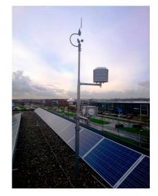
Figure 17. Weather station at the case study building.
