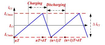
**Figure 6.** Capacitor current  $i_{C3}$ .
