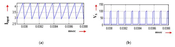
**Figure 15.** Simulation waveforms for input voltage 24V DC and 0.8 duty cycle; (**a**) input current waveform (current scale: 0.5 A/div and t: 20 μs/div) and (**b**) voltage across the power switch waveform (voltage scale 50 V/div and t: 20 μs/div).
