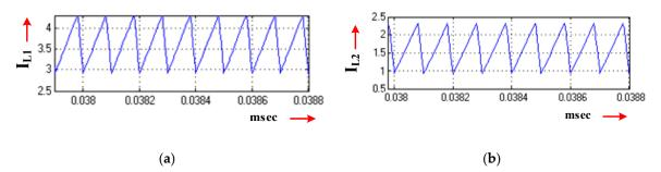
**Figure 16.** Simulation waveforms for input voltage 24 V DC and 0.8 duty cycle; (**a**) inductor current  $i_{L1}$  waveform (current scale: 0.5 A/div and t: 20  $\mu$ s/div) and (**b**) inductor current  $i_{L2}$  waveform (current scale: 0.5 A V/div and t: 20  $\mu$ s/div).
