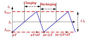
Figure 8. Evolution of the inductor current.
