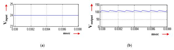
**Figure 14.** Simulation waveforms for input voltage 24V DC and 0.8 duty cycle; (a) input voltage waveform (voltage scale: 1 V/div and t:  $20 \mu s/div$ ) and (b) input voltage waveform (voltage scale 50 V/div and t:  $20 \mu s/div$ ).
