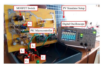
Figure 19. Prototype setup of the proposed converter.
