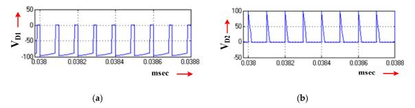
**Figure 17.** Simulation waveforms for input voltage 24V DC and 0.8 duty cycle; (**a**) voltage across the power diode,  $V_{D1}$  waveform (voltage scale: 50 V/div and t: 20  $\mu$ s/div) and (**b**) voltage across the power diode,  $V_{D2}$  waveform (voltage scale: 50 V/div and t: 20  $\mu$ s/div).
