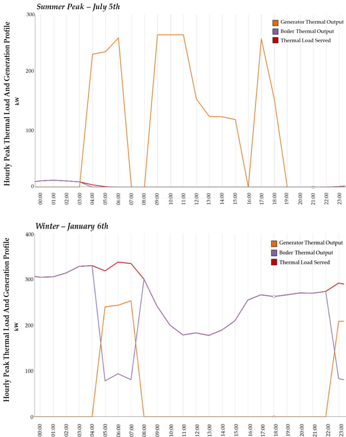
Figure 11. SHES dynamic thermal load management for a 150-persons base camp in Brandon, MB, in summer and winter peak days.
