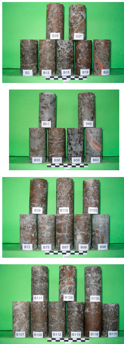
Figure A1. The Brown Zuber unit samples for short-term compression tests at a constant stress rate and for rheological tests.
