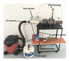
Figure 24. Prototype of combustion chamber used in experimental tests.
