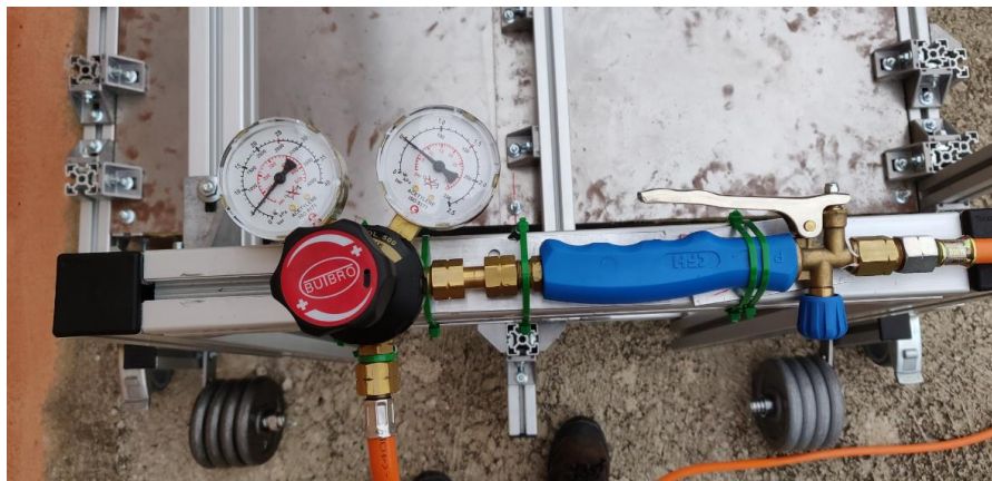
Figure 12. Manual pressure regulator and on/off valve.
