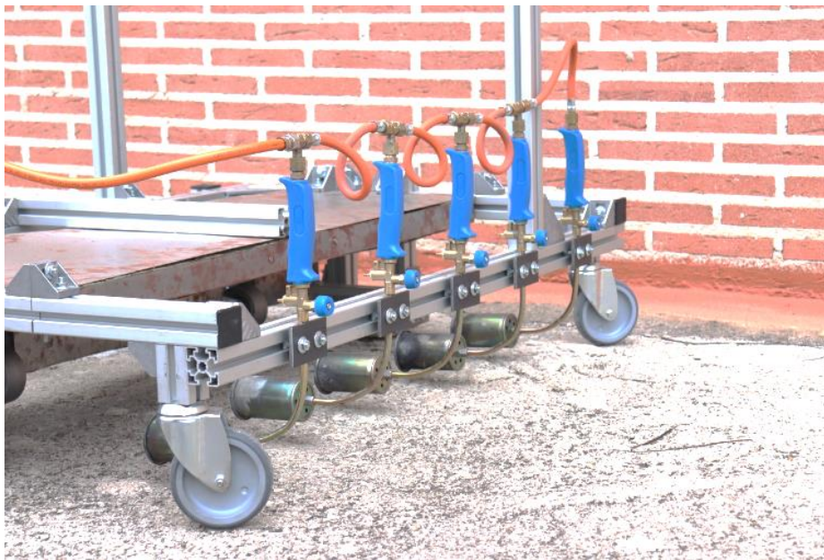
Figure 13. Individual flow regulators and parallel torches.
