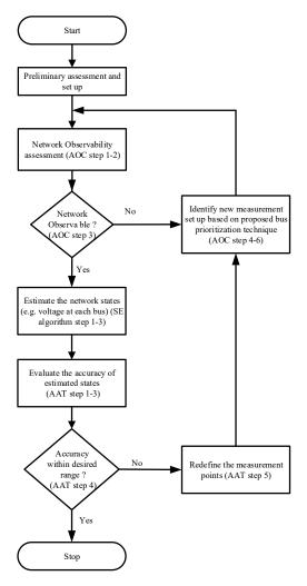
Figure 2. Compact algorithm for integrated assessment.
