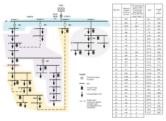
Figure 3. Modified MV network of Lind area, Denmark (observable islands in case 3).
