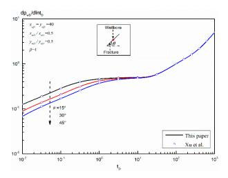
Figure 4. Validation of a finite-conductivity fracture with an azimuth angle in an anisotropic reservoir.
