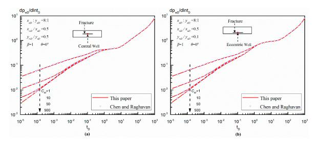
**Figure 3.** Validation of a fractured well located at different positions in an anisotropic rectangular reservoir. (**a**) central well; (**b**) eccentric well.
