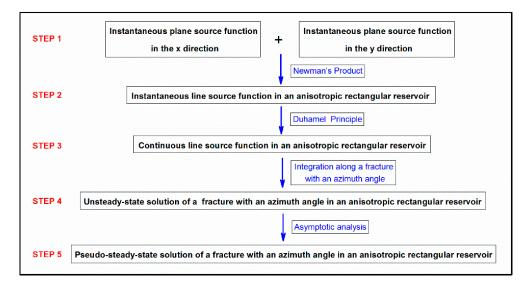
**Figure 2.** Derivation process of pseudo-steady-state solution of a fracture with an azimuth angle in an anisotropic rectangular reservoir.
