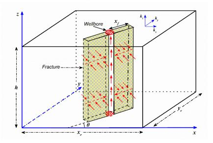
**Figure 1.** Schematic representation of a vertical well penetrated by a finite-conductivity fracture with an azimuth angle in an anisotropic rectangular reservoir.
