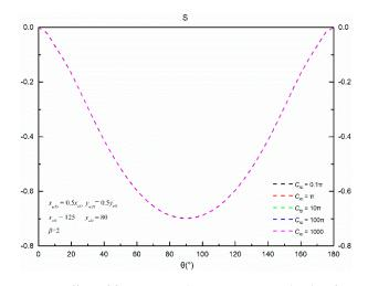
Figure 8. Effect of fracture conductivity on pseudo-skin factor.
