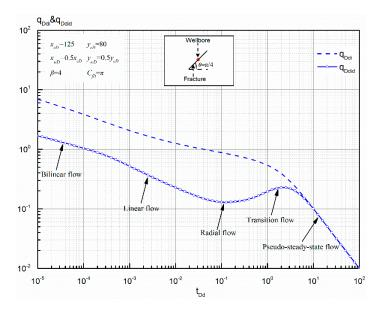
**Figure 12.** Flow regimes on Blasingame format curves for a well penetrated by a fracture with an azimuth angle in an anisotropic rectangular reservoir.
