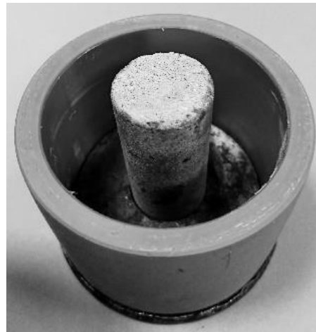
Figure 3. Core sample ready to be filled with cement slurry.
