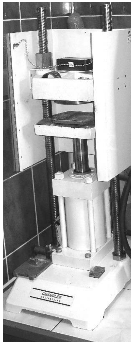
Figure 5. Machine for testing strength and adhesion.
