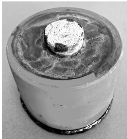
Figure 4. Sample prepared for adhesion tests.
