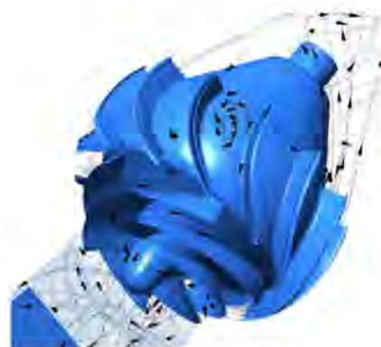
Figure 18. Suction and discharge recirculation caused by excessive swirl at the pump inlet bellmouth.
