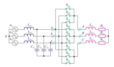
Figure 1. Matrix converter schematic diagram.
