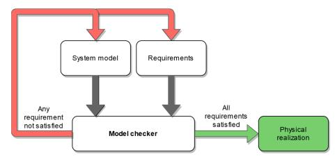
Figure 5. Process of symbolic model checking.
