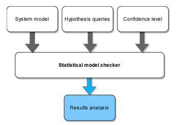
Figure 6. Process of statistical model checking.
