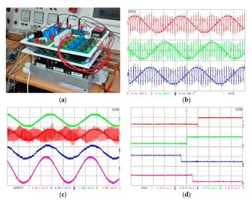
**Figure 4.** Low-power prototypes of Matrix Converter, (**a**) photo of power stage, (**b**) selected waveforms of three phase voltages, (**c**) selected waveforms of grid and loads voltages as well as source and loads currents, (**d**) transistor control waveforms for four-stage current commutation.
