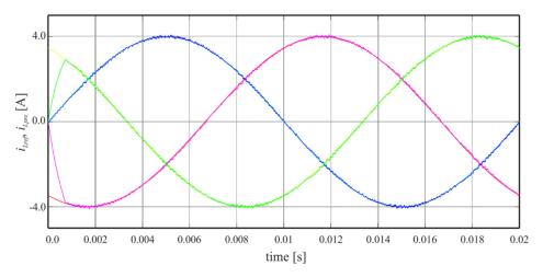
Figure 3. Output and reference currents in matrix converter using Simulink.
