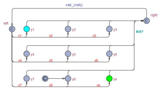
Figure 9. Abstract model of a controller in UPPAAL.
