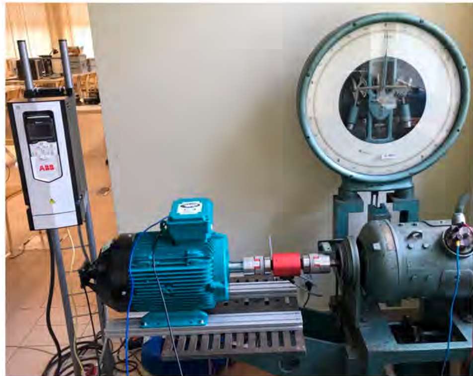
Figure 2. The tested motor (blue) with encoder on a test bench. In the upper left corner of the photo, there is an inverter that powers the motor. On the right is a loading DC generator and between machines is a torque meter (red).
