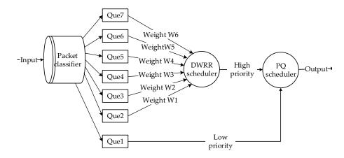
Figure 9. Algorithm principle diagram of PDWRR.
