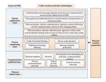
Figure 5. Cyber security protection system of SESt.
