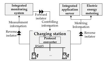
Figure 7. Isolation scheme between the charging station and other systems.
