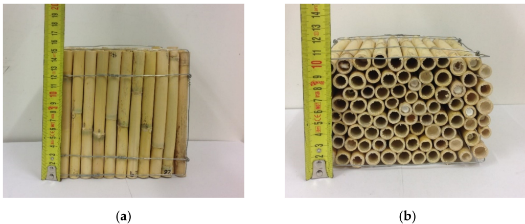
Figure 5. Reed panels used in hotbox test: (a) horizontal dimensions and (b) thickness.
