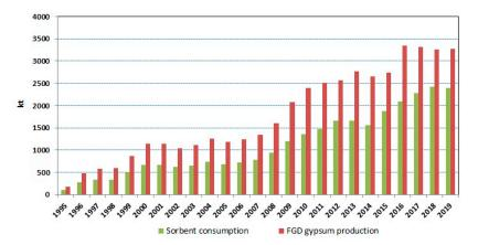
**Figure 1.** Comparison of the production volume of synthetic gypsum and consumption of limestone sorbents applied in flue gas desulphurisation in wet method (surveyed gypsum producers' and sorbent consumers' data).
