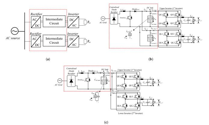
**Figure 1.** Schematic of: (**a**) the conventional parallel-connected system, (**b**) a multi-converter system with individual DC-bank having a centralized rectifier, (**c**) a multi-converter system with common DC-bank having a centralized rectifier
