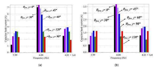
**Figure 6.** The  $f_{sw\_harmonic}$  = 40 kHz harmonic spectrum of capacitor bank current for various  $\theta_{fsw\_2}$  for the multi-converter system with: (a) common DC-bank, and (b) individual DC-banks—both at rated operating conditions.
