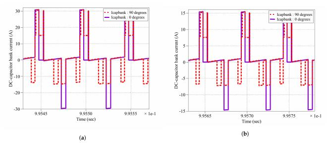
**Figure 7.** DC-capacitor bank current ripple reduction at  $\theta_{fsw_2} = 0^\circ$  (violet line), and  $\theta_{fsw_2} = 90^\circ$  (red dotted lines) for: (a) the multi-converter system with a common DC-bank, and (b) the multi-converter system with individual DC-banks.
