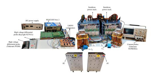
Figure 9. Experimental prototype of the multi-converter system.
