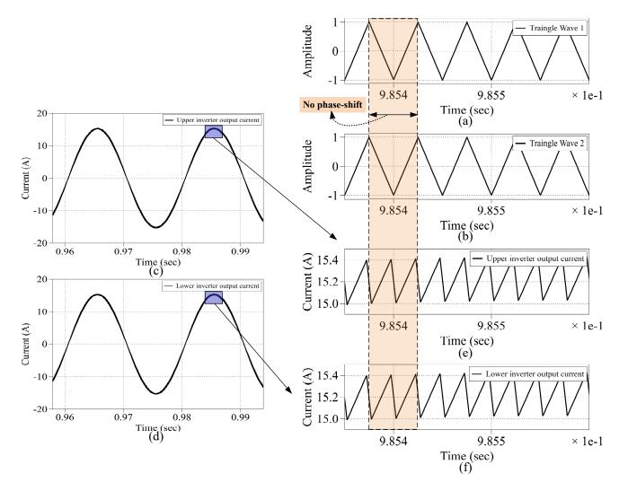
**Figure 5.** Parallel-connected system waves using the conventional method: (**a**) upper inverter carrier wave, (**b**) lower inverter carrier wave, (**c**) upper inverter output current wave, (**d**) lower inverter output current wave, (**e**) output current ripples of upper inverter, and (**f**) output current ripples of the lower inverter.
