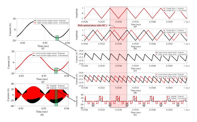
**Figure 8.** Red lines (proposed method with optimal phase-shift) and black lines (without any phase-shift): (**a**) upper inverter carrier wave, (**b**) lower inverter carrier wave, output current ripple of: (**c**) upper inverter, and (**d**) lower inverter, (**e**) total DC-capacitor current ripple, the time-domain waveform of output current from the: (**f**) upper inverter and (**g**) lower inverter, (**h**) total DC-capacitor current waveform.
