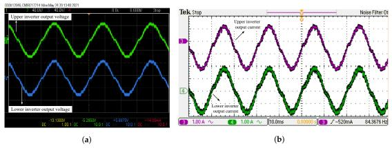
**Figure 11.** Measured waveforms of the multi-converter system with a common DC-bank (**a**) output voltages (**b**) output currents—two inverter units interleaved at  $\theta_{fsw_2} = 0^\circ$ , and  $\theta_{fsw_2} = 90^\circ$ , using parameters in Table 6.
