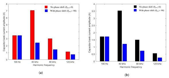
**Figure 12.** Effect of the optimal shift in the DC-capacitor bank current harmonics for: (**a**) the multi-converter system with a common DC-bank, (**b**) the multi-converter system with individual DC-banks.
