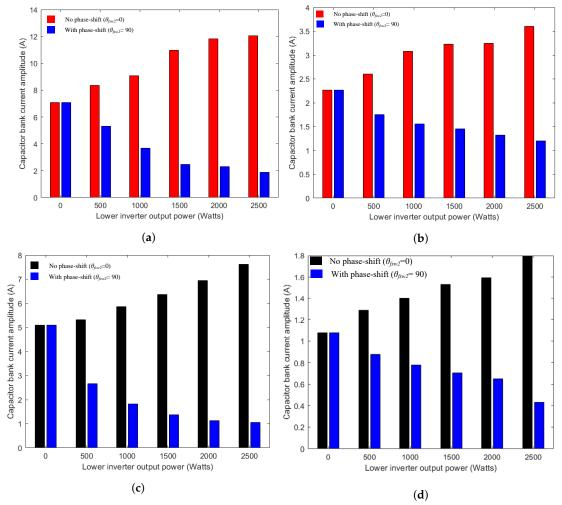
**Figure 13.** Effect of optimal shift in the DC-capacitor bank current for varying lower inverter loading in: the multi-converter system with a common DC-bank for (a)  $f_{sw\_harmonic} = 40$  kHz, (b)  $f_{sw\_harmonic} = 80$  kHz, and in the multi-converter system with individual DC-banks for (c)  $f_{sw\_harmonic} = 40$  kHz, (d)  $f_{sw\_harmonic} = 80$  kHz.
