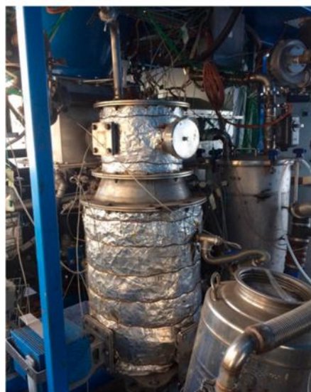
Figure 2. Downdraft gasifier developed by the C.M.D. company.
