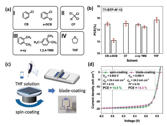
**Figure 4.** (a) Molecular formulas. (b) PCE histograms. (c) Schematics diagram of the spin-coating and blade-coating processes, and picture of the actual device. (d) The *J-V* curves of devices at a 1.07 cm<sup>2</sup> area. Reproduced from [55].
