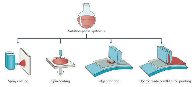
**Figure 1.** Different film preparation methods for solutions in the form of colloidal semiconductor inks. Reproduced from [3]. Reprinted with permission from ref. [3]. Copyright 2017 Nature Reviews Materials.
