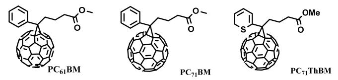
$\textbf{Figure 2.} \ \ \textbf{Representative chemical structures of fullerene derivatives}.$
