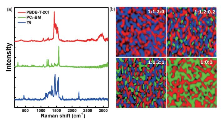
**Figure 8.** (a) Raman spectra of three materials: PBDB-T-2Cl, PC<sub>71</sub>BM and Y6; (b) Raman mapping image of ternary blend films with different PC<sub>71</sub>BM contents. Reproduced from [94]. Reprinted with permission from ref. [94]. Copyright 2019 Science China Chemistry.
