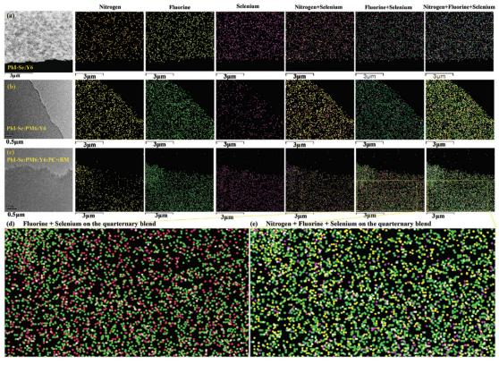
**Figure 12.** (**a–c**) Distribution of N, F and Se; (**d**,**e**) enlarged pictures. Reproduced from [51]. Reprinted with permission from ref. [51]. Copyright 2020 Wiley.
