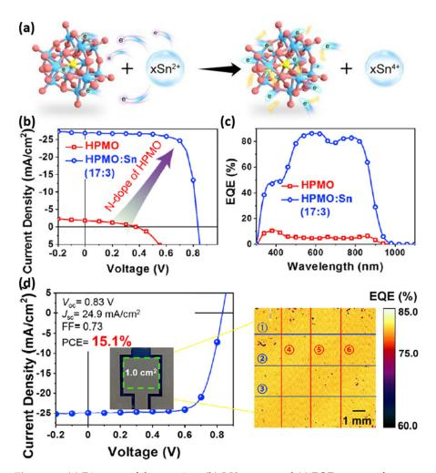
**Figure 14.** (a) Diagram of the reaction. (b) *J-V* curves and (c) EQE spectra of corresponding OPVs. (d) *J-V* curves and photovoltaic parameters of 1 cm<sup>2</sup> OPVs. Mapping image of EQE at 500 nm. Reproduced from [111]. Reprinted with permission from ref. [111]. Copyright 2021 Elsevier.
