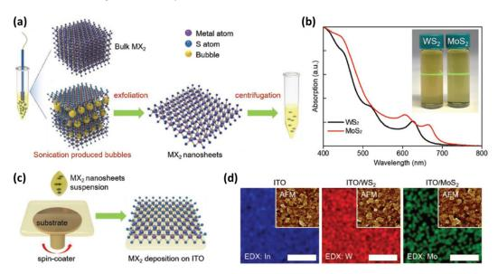
**Figure 13.** (a) The preparation process of  $MoS_2$  and  $WS_2$  suspensions. (b) Absorption spectra and the Tyndall effect in  $WS_2$  and  $MoS_2$  dispersions. (c) Schematic diagram of deposition of  $MoS_2$  and  $WS_2$  HTLs on substrate. (d) Element mapping obtained using EDX (scale bar: 2  $\mu$ m). Insets exhibit AFM images of corresponding samples. Reproduced from [33]. Reprinted with permission from ref. [33]. Copyright 2019 Wiley.
