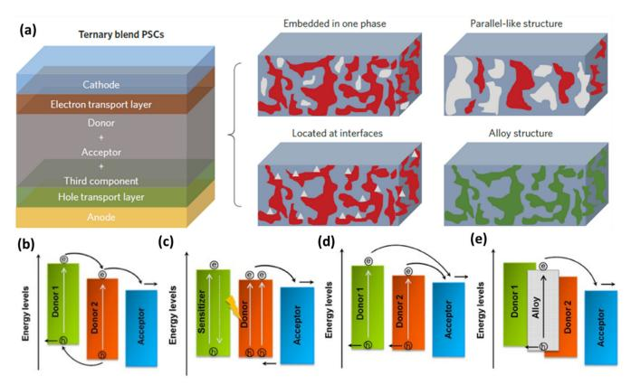
**Figure 7.** (a) Structures of ternary OPVs with four distribution patterns of the third component. Reproduced from [84]. Working principle diagram of ternary OPV based on double donors: (b) charge transfer, (c) energy transfer, (d) parallel-like mechanism and (e) alloy model. Reproduced from [90]. Reprinted with permission from ref. [84]. Copyright 2015 Nature Photonics; Reprinted with permission from ref. [90]. Copyright 2017 Wiley.
