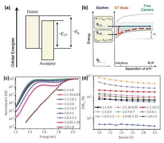
**Figure 10.** (a) Diagram of organic solar cell orbital energetics for a typical donor-acceptor pairing. (b) Schematic of two charge-generation pathways in systems with a large offset energy. Reproduced from [99]. (c) Normalized s-EQEs and (d) EQE<sub>EL</sub> values of the binary and ternary devices. Reproduced from [100].
