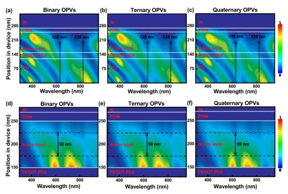
**Figure 11.** The simulated optical field distribution in the (a) binary, (b) ternary and (c) quaternary OPVs; calculated photogenerated exciton distribution in the optimized active layers of (d) binary, (e) ternary and (f) quaternary OPVs. Reproduced from [101]. Reprinted with permission from ref. [101]. Copyright 2020 Elsevier.
