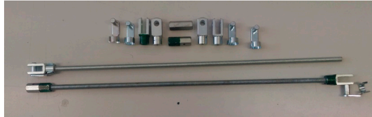
Figure 16. Bending pressure system set. Simple and economical system formed by two threaded rods with normal and reverse threads that allow us to achieve the necessary torque to bend the mirrors.
