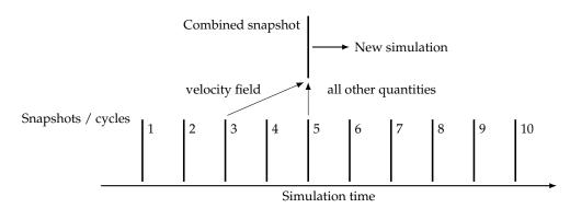
**Figure 1.** One possible combination of restart files: Here, the flow field is extracted from the third cycle and combined with all other quantities of the fifth cycle. The simulation then starts at the time when the fifth snapshot was taken.
