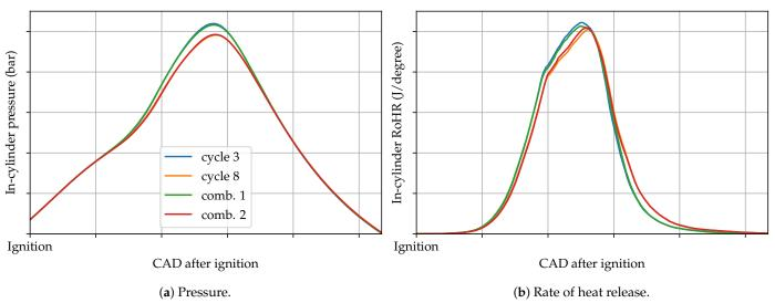
Figure 5. In-cylinder results for combinations 1 and 2.
