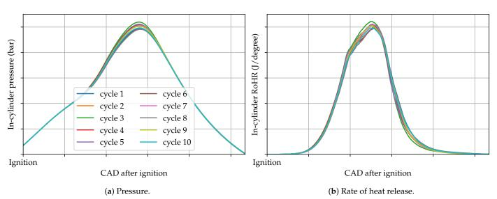
Figure 2. In-cylinder results for all ten cycles.
