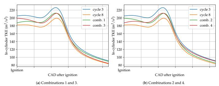
**Figure 7.** Average in-cylinder turbulent kinetic energy.
