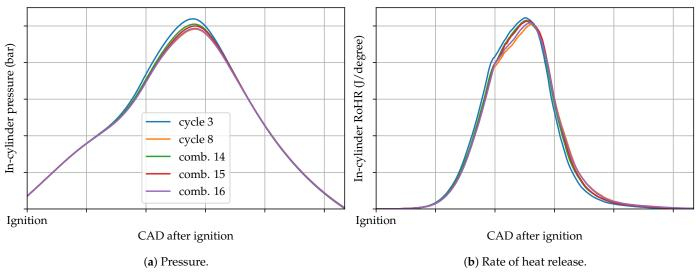
**Figure 11.** In-cylinder results for combinations 14, 15 and 16.
