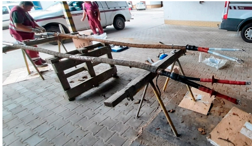
Figure 10. The samples preparation, assembly of termination before sending for testing.
