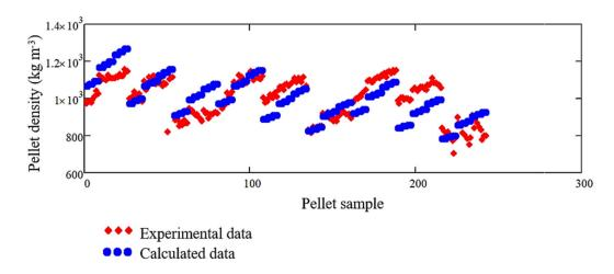
Figure 7. Graphical comparison between the data calculated using relation (15) and the experimental data for the 10 mm die.
