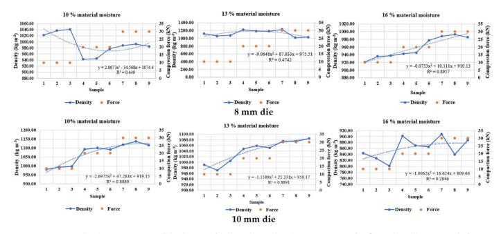
**Figure 16.** Graphical representation of the density of pellets obtained at the temperature of 70  $^{\circ}$ C and a pelleting speed of 2.8 mm s<sup>-1</sup> for the three moistures used.
