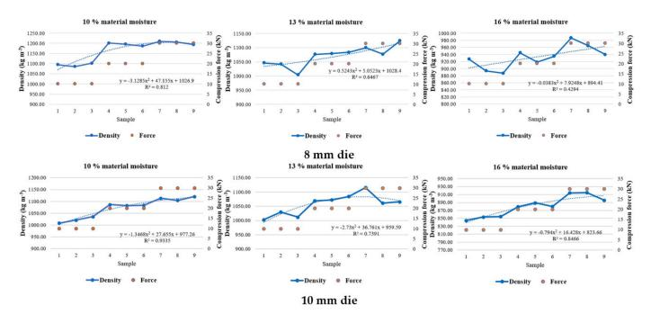
**Figure 14.** Graphical representation of the density of pellets obtained at the temperature of 90  $^{\circ}$ C and a pelleting speed of 2.1 mm s<sup>-1</sup> for the three moistures used.
