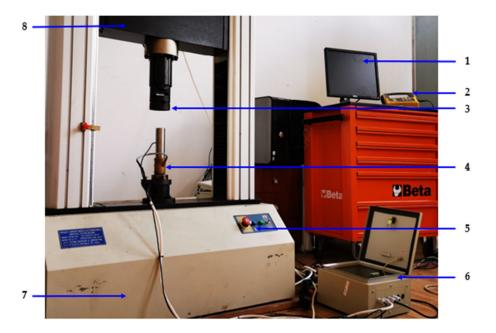
**Figure 2.** Force machine connected to the pelleting device. 1. computer; 2. phase and frequency analyzer; 3. pressing head; 4. pelleting device; 5. force machine control panel; 6. automation box; 7. casing; 8. pressing support.
