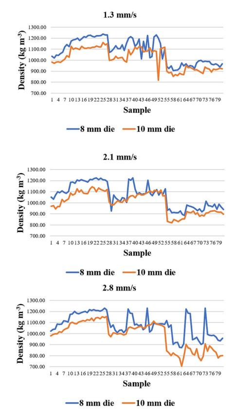
**Figure 11.** Comparisons between the variation of pellet density depending on the pelleting speed for the two dies used.
