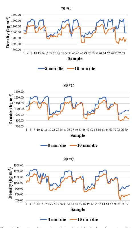
**Figure 12.** Comparisons between the variation of pellet density depending on the pelleting temperature for the two dies used.
