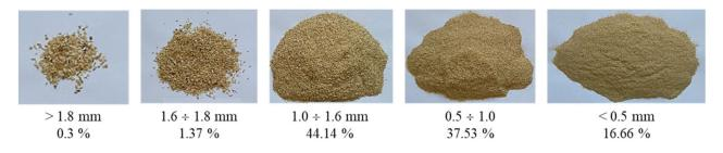
Figure 4. Fir sawdust measuring <2 mm separated on fractions.
