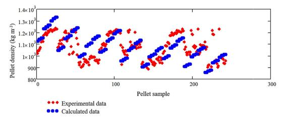
Figure 6. Graphical comparison between the data calculated using relation (15) and the experimental data for the 8 mm die.
