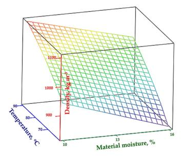
**Figure 8.** Pellet density dependency on initial sawdust moisture and on the temperature reached in the pelleting die.
