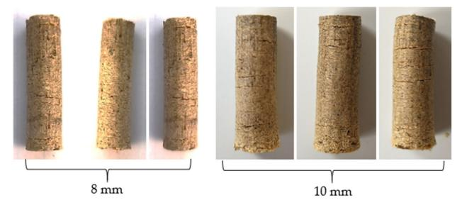
Figure 5. Pellet samples obtained from fir sawdust.
