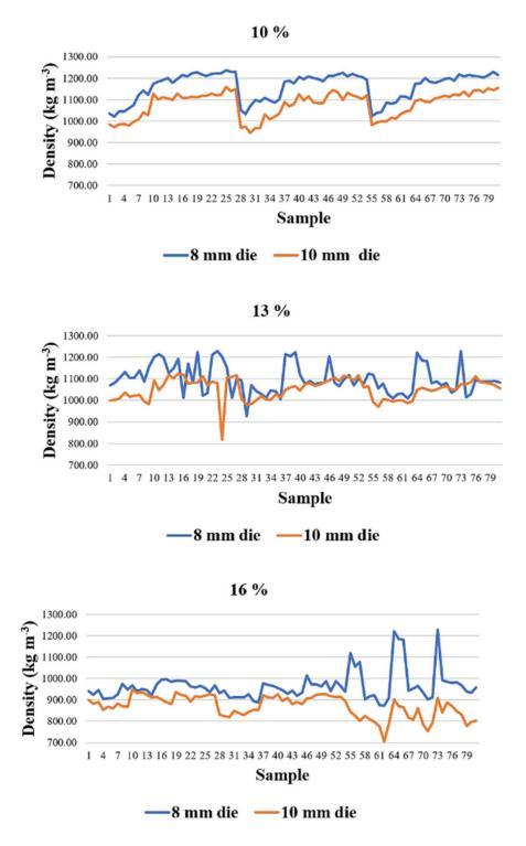
**Figure 9.** Comparisons between the variation of pellet density depending on the initial moisture of the raw material, for the two dies used.
