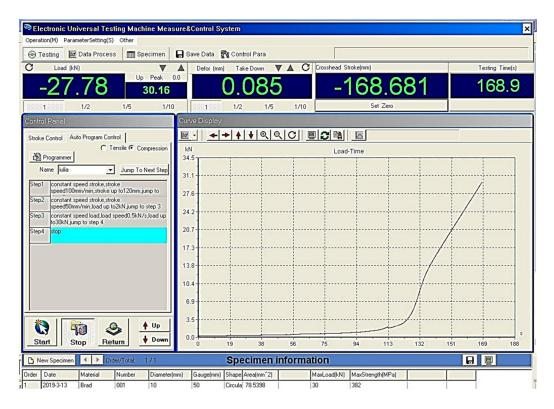
Figure 3. Time-force curve generated by the software for a pelleting sample.
