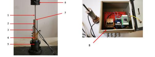
**Figure 1.** Pelleting device used for experiments. 1. piston; 2. interchangeable die (8, 10 mm for the pelleting orifice); 3. temperature sensor; 4. heating element; 5. blocking plate; 6. pressing head; 7. pelleting orifice; 8. automation box.
