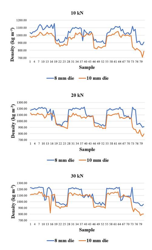
**Figure 10.** Comparisons between the variation of pellet density depending on the compression force for the two dies used.
