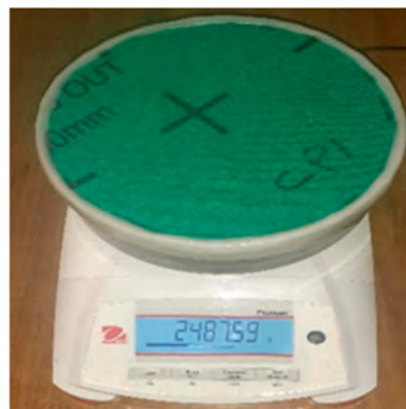
Figure 5. Weighing of cup assembly.
