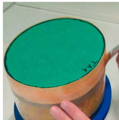
Figure 4. Taping and wax sealing.
