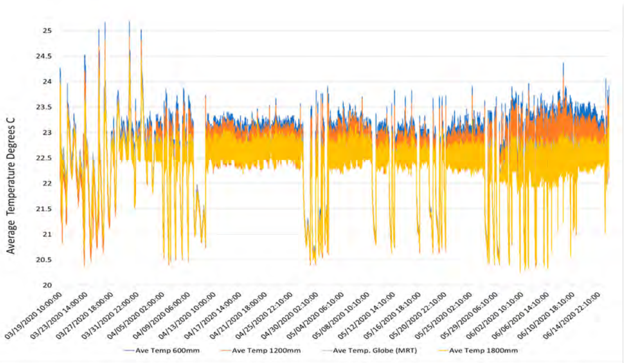
Figure A1. Temperature profile of the hygrothermal room aimed at 23 °C for the testing period 1.
