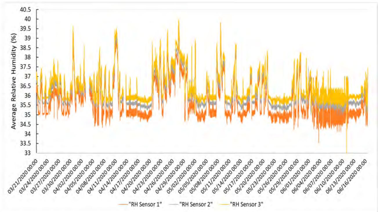
Figure A5. Relative humidity profile of the room aimed at 35% for the testing period 1.
