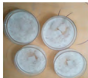
Figure 2. Glass dishes for wet cup test with saturated ammonium dihydrogen phosphate.
