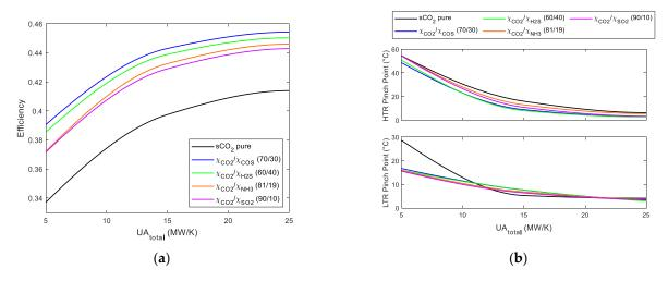
**Figure 11.** (a) Cycle efficiency vs.  $UA_{total}$ . RCC with four reheatings Brayton cycles using s-CO<sub>2</sub> mixtures. (b) LTR and HTR pinch point vs.  $UA_{total}$ . RCC with four reheatings Brayton cycles using s-CO<sub>2</sub> mixtures.
