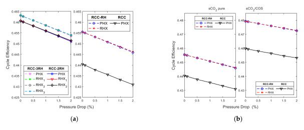
**Figure 16.** Cycle efficiency vs. pressure drop. (a) RCC, RCC-RH, RCC-2RH, and RCC-3RH Brayton cycle using s-CO<sub>2</sub> pure and  $UA_{total} = 15 \text{ MW/K}$ . (b) RCC and RCC-RH Brayton cycle using mixtures s-CO<sub>2</sub>/COS and  $UA_{total} = 15 \text{ MW/K}$ .
