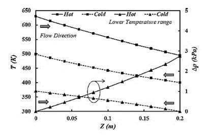
**Figure 22.** Temperature variation (left ordinate) and pressure drop (right ordinate) of the straight channel along the length for the lowest temperature range in the comparison study.
