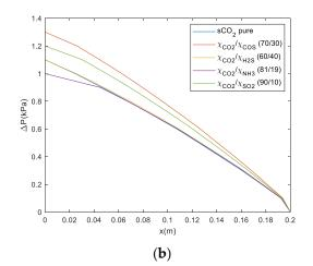
Figure 19. Pressure drop of the different s-CO<sub>2</sub> mixtures in the straight channels; (a) hot fluid; (b) cold fluid.
