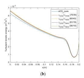
Figure 20. Turbulent kinetic energy of the different mixtures in the straight channels; (a) hot fluid, (b) cold fluid.
