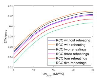
Figure 6. Cycle efficiency vs. UA<sub>total</sub>. RCC Brayton cycles using pure s-CO<sub>2</sub> with pressure drop.
