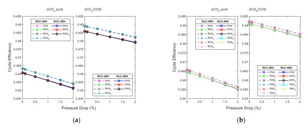
**Figure 17.** Cycle efficiency vs. pressure drop. (a) RCC-2RH and RCC-3RH Brayton cycle using mixtures s-CO<sub>2</sub>/COS and UA<sub>total</sub> = 15 MW/K. (b) RCC-4RH and RCC-5RH Brayton cycle using mixtures s-CO<sub>2</sub>/COS and UA<sub>total</sub> = 15 MW/K.
