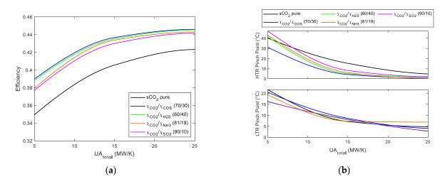
**Figure 7.** (a) Cycle efficiency vs.  $UA_{total}$ . RCC without reheating Brayton cycles using s-CO<sub>2</sub> mixtures. (b) LTR and HTR pinch point vs.  $UA_{total}$ . RCC without reheating Brayton cycles using s-CO<sub>2</sub> mixtures.
