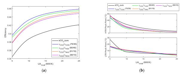
**Figure 10.** (a) Cycle efficiency vs.  $UA_{total}$ . RCC with three reheatings Brayton cycles using s-CO<sub>2</sub> mixtures. (b) LTR and HTR pinch point vs.  $UA_{total}$ . RCC with three reheatings Brayton cycles using s-CO<sub>2</sub> mixtures.
