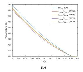
Figure 18. Temperature profile of the different mixtures; (a) hot fluid; (b) cold fluid.
