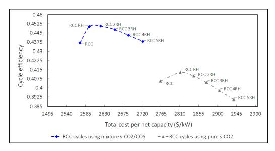
**Figure 25.** Cycle efficiency vs. total cost per net capacity of the RCC Brayton cycles using pure s- $CO_2$  and mixture s- $CO_2$ /COS (70/30) with pressure drop.
