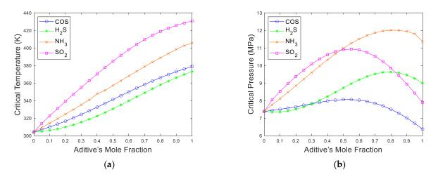
Figure 2. Fluids properties vs. additive's mole fraction. (a) Critical temperature, (b) critical pressure.
