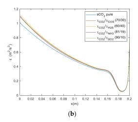
**Figure 21.** Dissipation rate of the different mixtures' turbulent kinetic energy in the straight channels; (a) hot fluid, (b) cold fluid.
