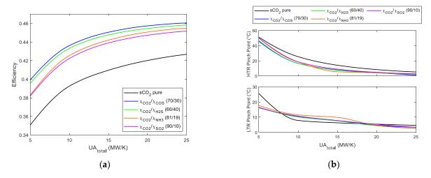
**Figure 9.** (a) Cycle efficiency vs.  $UA_{total}$ . RCC with two reheatings Brayton cycles using s-CO<sub>2</sub> mixtures. (b) LTR and HTR pinch point vs.  $UA_{total}$ . RCC with two reheatings Brayton cycles using s-CO<sub>2</sub> mixtures.
