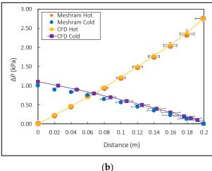
**Figure 23.** (a) Comparison between reference temperature values and the values obtained in the simulation; (b) Comparison between reference pressure drop values and the values obtained in the simulation.
