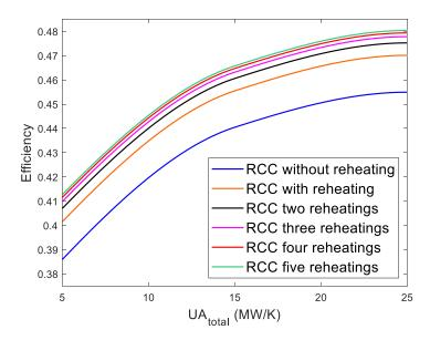
Figure 3. Cycle efficiency vs. UA<sub>total</sub>. RCC Brayton cycles using pure s-CO<sub>2</sub> without pressure drop.
