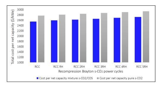
**Figure 24.** Comparisons of total cost net per capacity of the RCC Brayton cycles using pure s- $CO_2$  and mixture s- $CO_2$ /COS (70/30).
