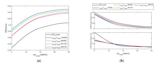
**Figure 12.** (a) Cycle efficiency vs.  $UA_{total}$ . RCC with five reheatings Brayton cycles using s-CO<sub>2</sub> mixtures. (b) LTR and HTR pinch point vs.  $UA_{total}$ . RCC with five reheatings Brayton cycles using s-CO<sub>2</sub> mixtures.
