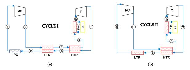
Figure 15. Division into two parts of the recompression Brayton s-CO<sub>2</sub> power cycle. (a) Cycle I and (b) Cycle II.
