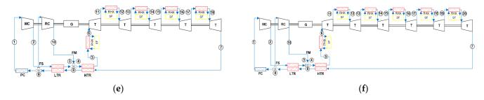
**Figure 1.** Layout of recompression Brayton cycle (a), with reheating (b), with two reheatings (c) with three reheatings (d), with four reheatings (e), and with five reheatings (f). MC: main compressor; RC: recompressor; G: generator; T: turbine; PC: precooler; FS: fluid split; FM: fluid mixture; LTR: low-temperature recuperator; HTR: high-temperature recuperator; PHX: primary heat exchanger; RHX: reheating heat exchanger; SF: solar field.
