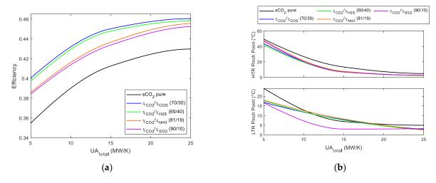
**Figure 8.** (a) Cycle efficiency vs. UA<sub>total</sub>. RCC with reheating Brayton cycles using s-CO<sub>2</sub> mixtures. (b) LTR and HTR pinch point vs. UA<sub>total</sub>. RCC with reheating Brayton cycles using s-CO<sub>2</sub> mixtures.
