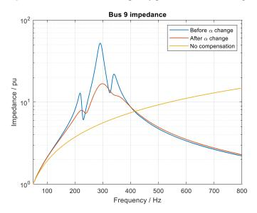
Figure 16. The 7th harmonic frequency parallel resonance mitigation in bus 9.
