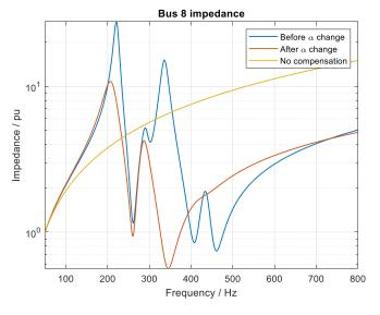
Figure 15. The 7th harmonic frequency parallel resonance mitigation in bus 8.
