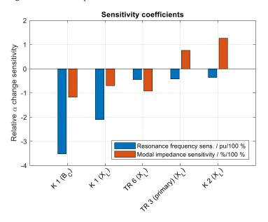
Figure 12. Resonance sensitivity coefficients of mode 5 (bus 6 is short-circuited.).
