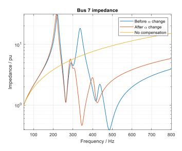
Figure 14. The 7th harmonic frequency parallel resonance mitigation in bus 7.
