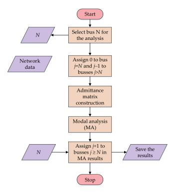
Figure 3. Series resonance network topology modification algorithm.
