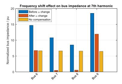
**Figure 17.** Comparison of the impedances of busses 6, 7, 8 and 9 before and after the series frequency shift.
