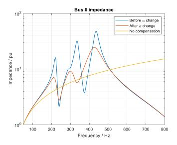
Figure 13. The 7th harmonic frequency parallel resonance mitigation in bus 6.
