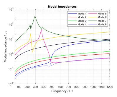
Figure 11. Modal impedances of the network with short-circuited bus 6.
