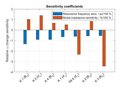
Figure 7. Resonance sensitivity coefficients of mode 5.
