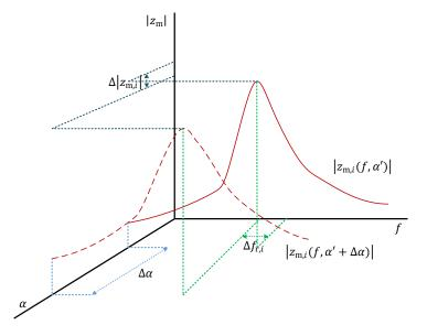
Figure 2. Network parameters change effect on a modal impedance characteristic.
