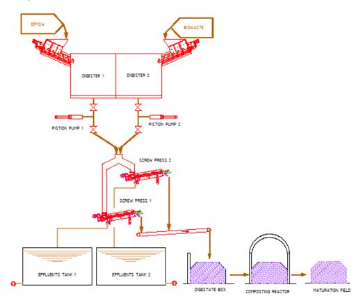
Figure 1. Simplified diagram of the biological treatment facility.
