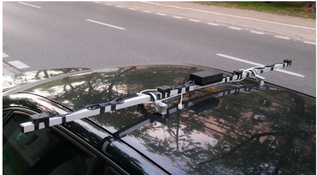
Figure 4. View of the proprietary measurement system on the vehicle roof.
