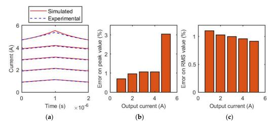
**Figure 10.** Coilcraft MSS1260T-273 inductor, 12 V. (a) Comparison of experimental and simulated current waveforms for different output current values; (b) relative error of the estimation of the peak value of the inductive current; (c) relative error of the estimation of the RMS value of the inductive current.
