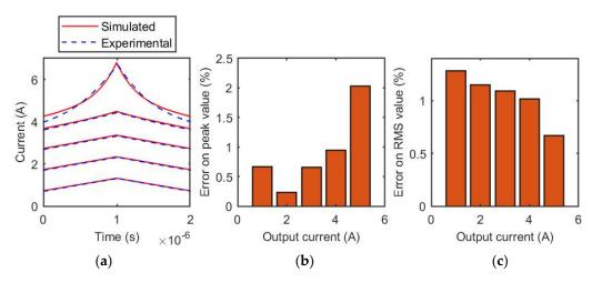
**Figure 11.** Coilcraft MSS1260T-273 inductor, 32 V. (a) Comparison of experimental and simulated current waveforms for different output current values; (b) relative error of the estimation of the peak value of the inductive current; (c) relative error of the estimation of the RMS value of the inductive current.
