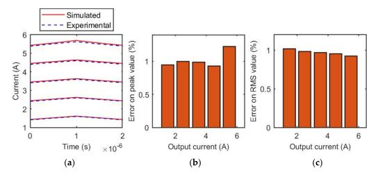
**Figure 15.** Coilcraft SER1390-333 inductor, 12 V. (a) Comparison of experimental and simulated current waveforms for different output current values; (b) relative error of the estimation of the peak value of the inductive current for each tested output current value; (c) relative error of the estimation of the RMS value of the inductive current for each tested output current value.
