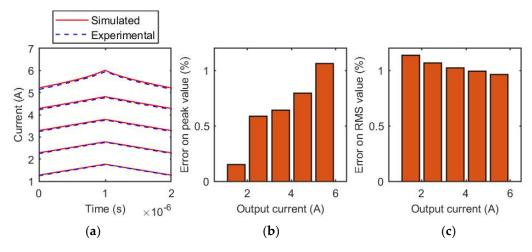
**Figure 16.** Coilcraft SER1390-333 inductor, 32 V. (a) Comparison of experimental and simulated current waveforms for different output current values; (b) relative error of the estimation of the peak value of the inductive current for each tested output current value; (c) relative error of the estimation of the RMS value of the inductive current for each tested output current value.
