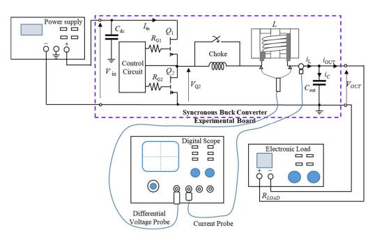
Figure 1. Circuit diagram of the experimental setup for DC thermal steady-state differential inductance identification. A high inductance choke allows imposing negligible current ripple on the inductor under test. After reaching the DC thermal steady-state for a given average output current, the choke is short-circuited, and the inductor voltage and current waveforms are measured with a digital oscilloscope.
